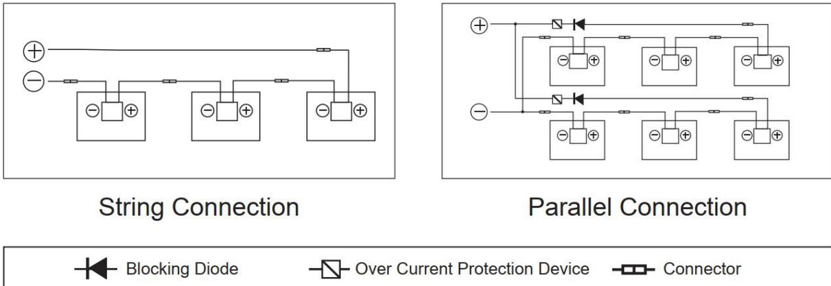
Figure 11 Series connection and parallel connection circuit diagram
