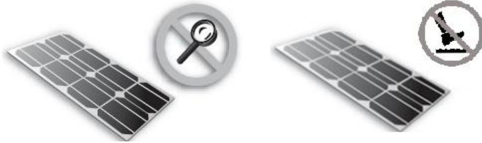
1.2.9 Avoid moving the modules by pulling cables or the junction box.
