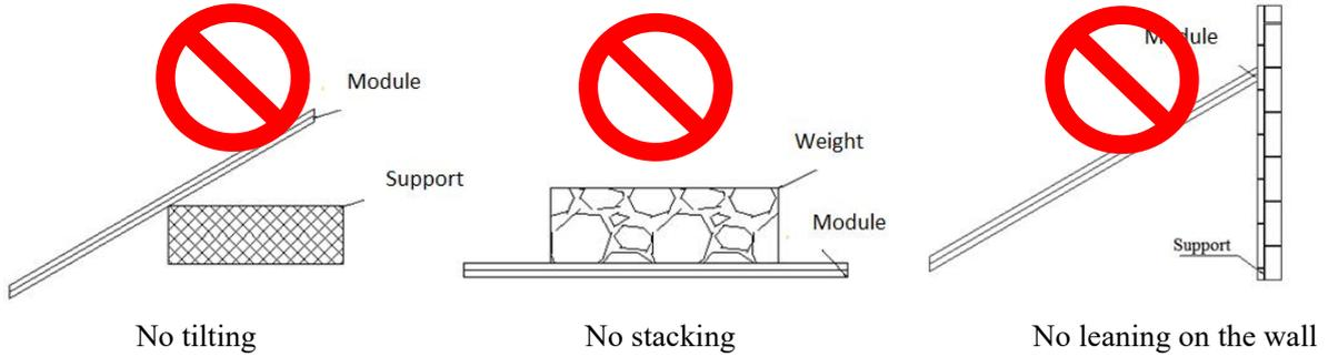
Figure 5 Modules stack illustration
