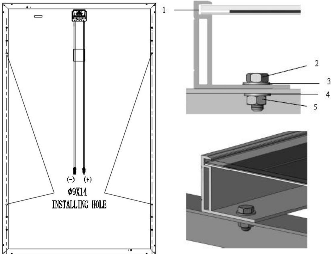
Figure 7. SPV module installed with Bolt fitting method
